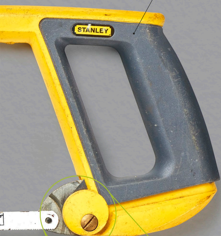
Quick-release lever pivots around screw.
