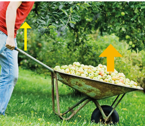
A wheelbarrow is a class 2 lever. It magnifies the weak force from your arms to pick up the heavy load.
