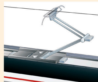
The train's metal arm is called a pantograph.
