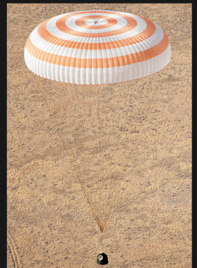
The Soyuz descent module slows down as it falls through Earth's atmosphere, and a parachute slows it even more, so that the astronauts inside can land safely.
