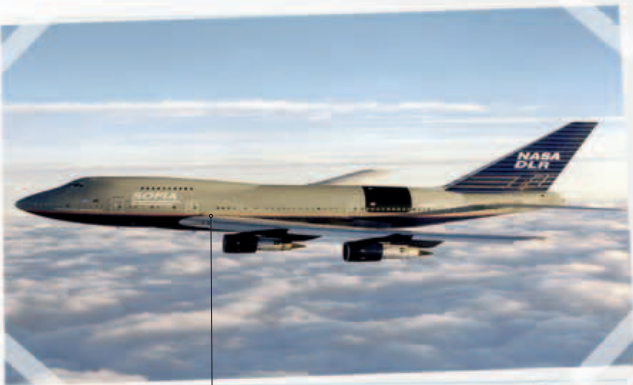
Aircraft houses an 8 ft (2.5 m) wide infrared telescope.
