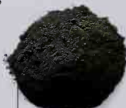
ALUMINUM Powder coated with aluminum oxide, \text{Al}_2\text{O}_3
