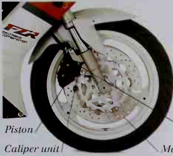
Brake pad (inside caliper unit) Metal brake disk
