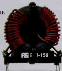
INDUCTOR FOR BLOCKING CURRENT INTERFERENCE
