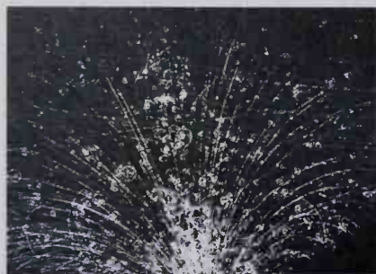
Tracks left by cosmic rays in a bubble chamber
