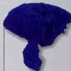
COPPER(II) NITRATE Copper(II) nitrate is hygroscopic, which means that it absorbs water from the air
