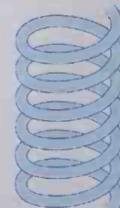
HELIX A twisted curve. The distance moved in one revolution is its pitch.
