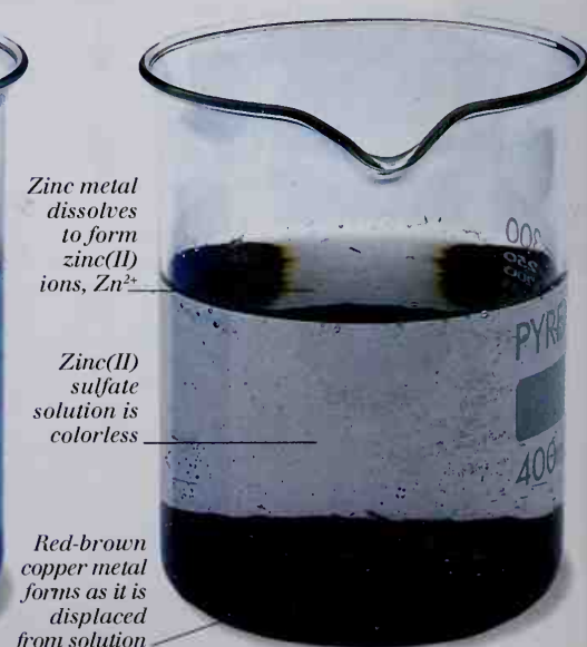
ZINC(II) SULFATE SOLUTION AND METALLIC COPPER
