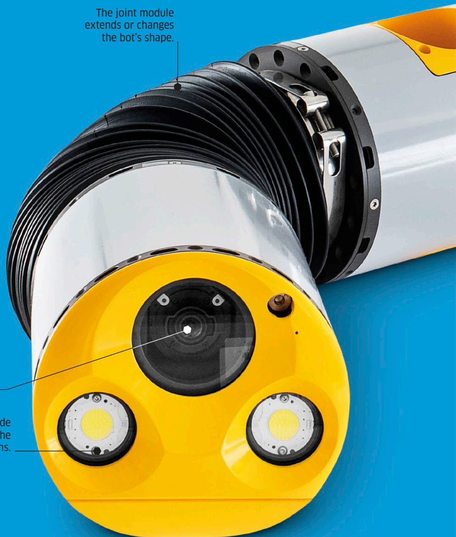
The front-facing HD camera can capture crystal-clear photographs and video footage.
