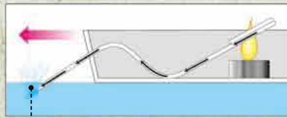
Steam jets out of the tube, pushing the boat forward
