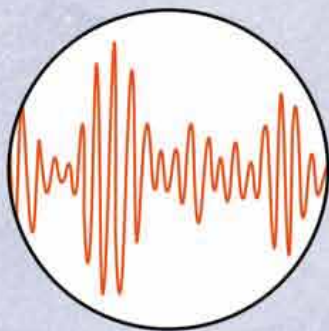
Sound wave changes the amplitude of the carrier wave
