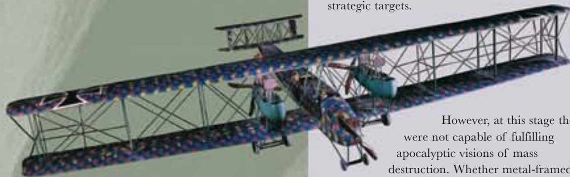
SHADOW OVER THE WESTERN FRONT The Zeppelin Staaken R.IV, of which the above is a model, flew on the Western Front in 1917–18. This six-engined monster had a wingspan of 42.2m (138ft 6in) and, when fully loaded, weighed over 13 tonnes (almost 13 tons).
