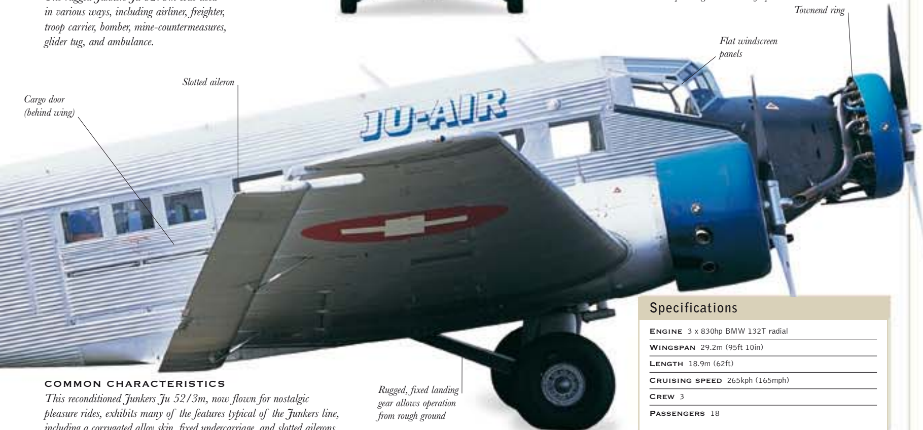
Auxiliary flying surface, incorporating ailerons and flaps
