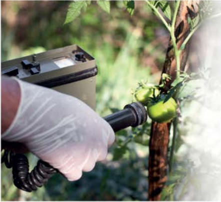
Measuring radiation levels in tomatoes
