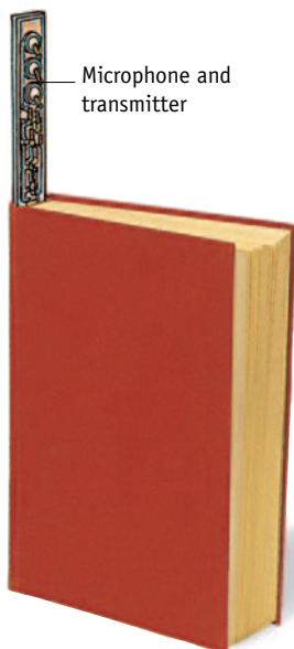
INSERTION OF TRANSMITTER INTO BOOK SPINE
