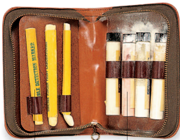
Invisible crayon for sticking the powder to a surface
