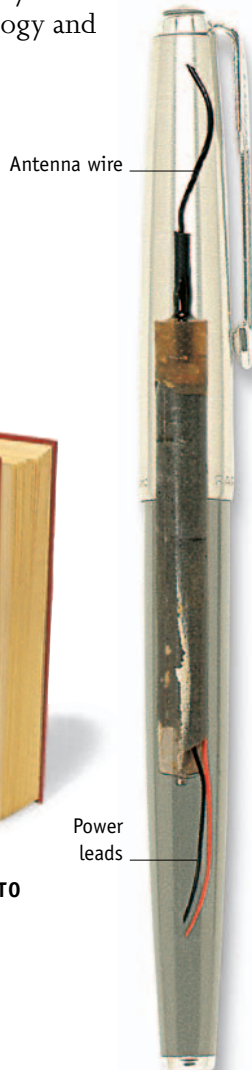
MICROPHONE AND TRANSMITTER CONCEALED IN PEN
