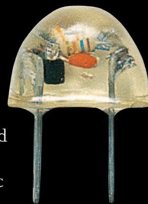
CIA infrared receiver This small device was plugged into an electrical socket and controlled remotely to trigger a hidden surveillance camera.
