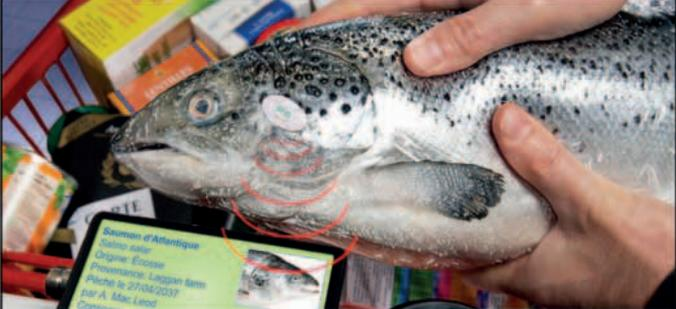
Radio frequency identification (RFID) is likely to take over some of the tasks that bar codes perform today. This image shows how the system might work: a radio-tagged salmon is being checked out on a “smart” supermarket trolley.
