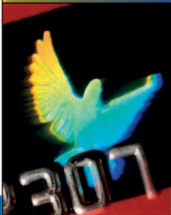
Holograms are pictures that appear in 3-D (three-dimensional). Making a hologram involves lasers, beam splitters, lenses, mirrors, and special film. Holograms make it very difficult to produce fake copies of credit cards.
