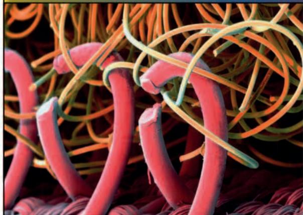
One backing surface is packed with countless tufts of fine nylon loops. On the other surface, there is a heavier grade of nylon, which is sewn and then cut under hot infrared lights to form hooks. Each piece can be used again and again, because there are so many hooks and loops, which fasten to form a bond.
