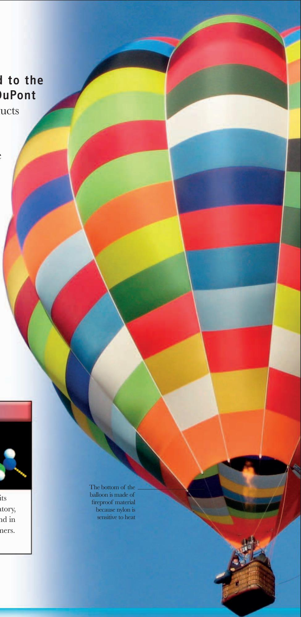
The bottom of the balloon is made of fireproof material because nylon is sensitive to heat
