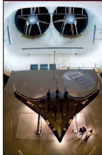
The X-48B Boeing Phantom is a type of experimental plane based on a flying wing design. This means that the entire plane is designed to act as a single huge wing, all of which provides an upward thrust on the plane. However, the shape of these experimental planes makes them difficult for pilots to control.
