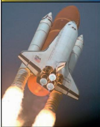
Rockets work because they follow Isaac Newton's third law of motion: each force (an action) has an equal force in the opposite direction (the reaction). As the fuel burns, the expanding exhaust gases are pushed backward, and the Newtonian reaction pushes the rocket forward.
