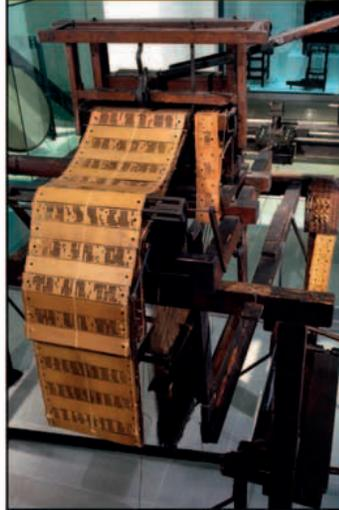
Like a robot, the Jacquard loom followed coded instructions, but while modern robots receive instructions from computers, the loom was controlled by cards with holes punched in them. These directed the positions of the threads, so different patterns could be woven automatically. It was invented in 1801 by Joseph-Marie Jacquard.
