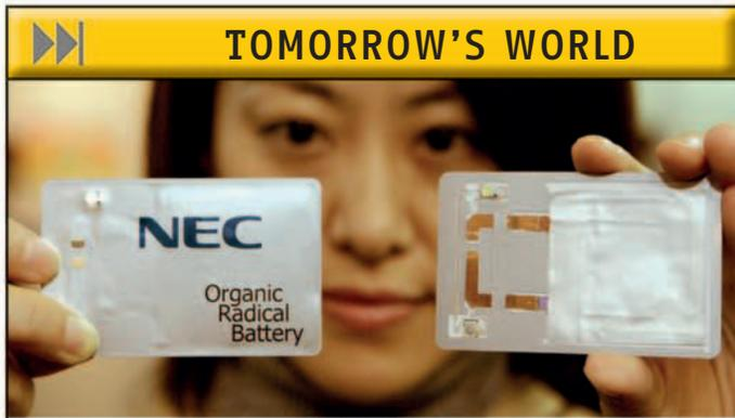
These organic radical batteries are bendable, less than  $\frac{1}{25}$  in (1 mm) thick, and are fully charged in less than 30 seconds. They do not use harmful metal chemicals to make electricity, so they can be safely thrown away.
