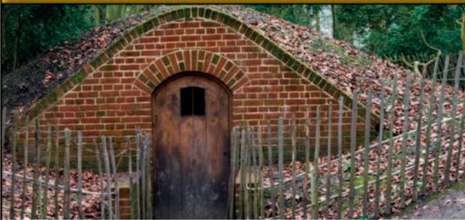
Until the mid-1900s, people moved natural ice from cold parts of the world to warmer areas and stored them in underground “ice houses.” Chunks of ice from the ice houses were used to cool “iceboxes,” which were like unpowered refrigerators.
