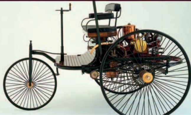
The world’s first car, the three-wheeler Benz Motorwagen designed by German engineer Karl Benz, took to the road in 1886. Its most famous trip was made in 1888, when the inventor’s wife drove it nearly 124 miles (200 km) at a top speed of 10 mph (16 km/h).
