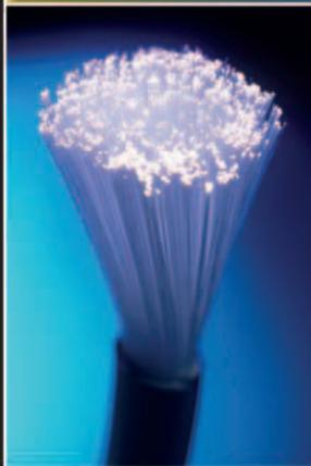
When light enters one end of an optical fiber, it stays inside the fiber. Even if the fiber is bent or tied in a knot, the light stays inside it and follows it to the end, like water flowing through a bent pipe. Optical fibers have to be made of very pure glass, free from defects, in order to carry the maximum light intensity from end to end.
