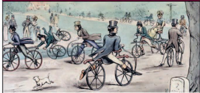
First demonstrated in 1818, Baron Karl Drais von Sauerbronn's wooden *Laufmaschine* (running machine) was one of the world's first bicycles. With no pedals, riders pushed their feet against the ground to roll forward.
