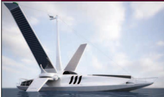
Volitan ("Flying fish") is an innovative sailboat that shows the way future vessel designs can use environmentally friendly features. With its solid solar-panel covered sails, Volitan uses both wind power and solar energy.
