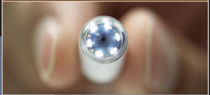
An endoscope the size of a large pill has been developed. Called a capsule endoscope, it is swallowed by a patient and passes through the body, transmitting pictures on its way. Future capsule endoscopes may be self-propelled and able to carry out minor surgery using a movable arm.
