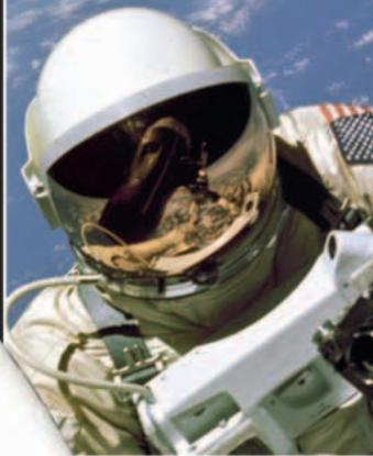
Early space helmets fogged up when astronauts worked hard: their breath formed a mist on the faceplate. Later helmets used air flow and antifog spray to keep them clear. They also had dark visors to protect astronauts' eyes from the dazzling glare of bright sunlight.
