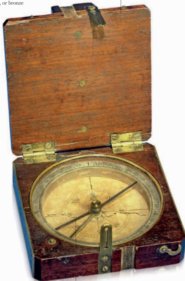
A magnetized needle pivots on top of a sharp point
