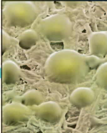
The glue contains billions of tiny sticky acrylic spheres; the gaps between the spheres prevent them from sticking too well. A coating on the back of the notes makes the glue stay on them and not transfer to the other surface.
