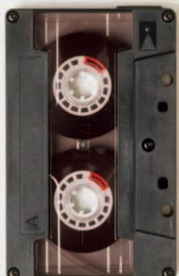
A cassette contains plastic tape with magnetically charged particles. The tape passes over a playing head, which reacts with the magnetic particles. This creates vibrations that are converted into sound by the headphone speakers.
