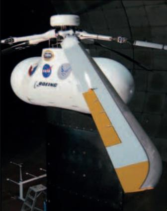
Helicopters use a lot of fuel. They also make a lot of noise. Scientists, however, are developing new types of helicopter blades that change shape when electrical signals are fed to them. This makes them move through the air more quietly, and means less fuel is needed, too.
