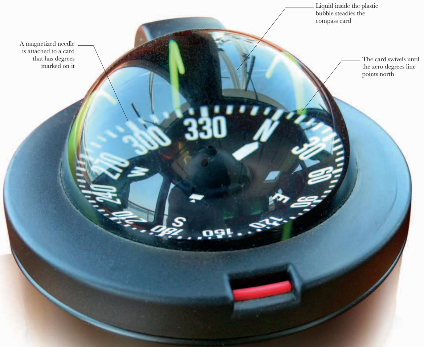
A magnetized needle is attached to a card that has degrees marked on it
