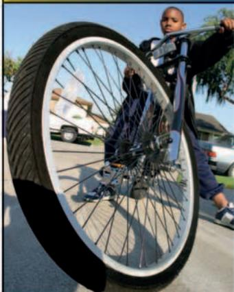
Spokes make wheels lighter, while keeping their strength. On wooden wheels the spokes push outward, but bicycles have wire spokes that pull inward. The advantage of these is that the wheel can change shape slightly without breaking.
