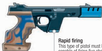
Ammunition propulsion The ammunition is propelled by precompressed air or by a carbon dioxide cylinder
