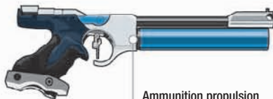
Ammunition propulsion The ammunition is propelled by precompressed air or by a carbon dioxide cylinder
