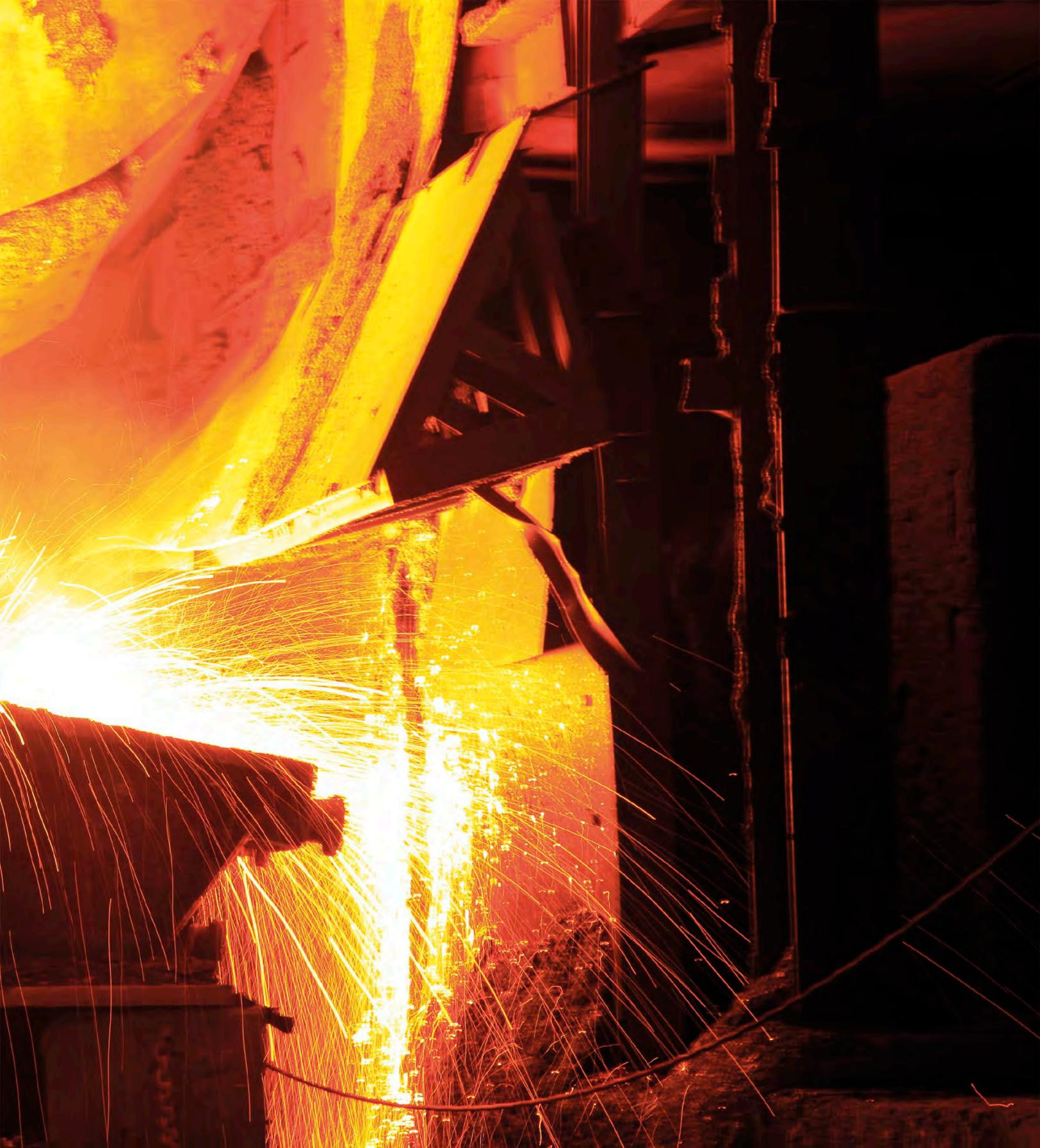
Steel is an alloy of iron that contains about two per cent carbon and some other elements. The carbon locks all the atoms together and prevents the metal from cracking. This makes steel harder than iron: it bends before it breaks and doesn't shatter easily. To make steel, iron ore is smelted in a blast furnace to remove its impurities,
