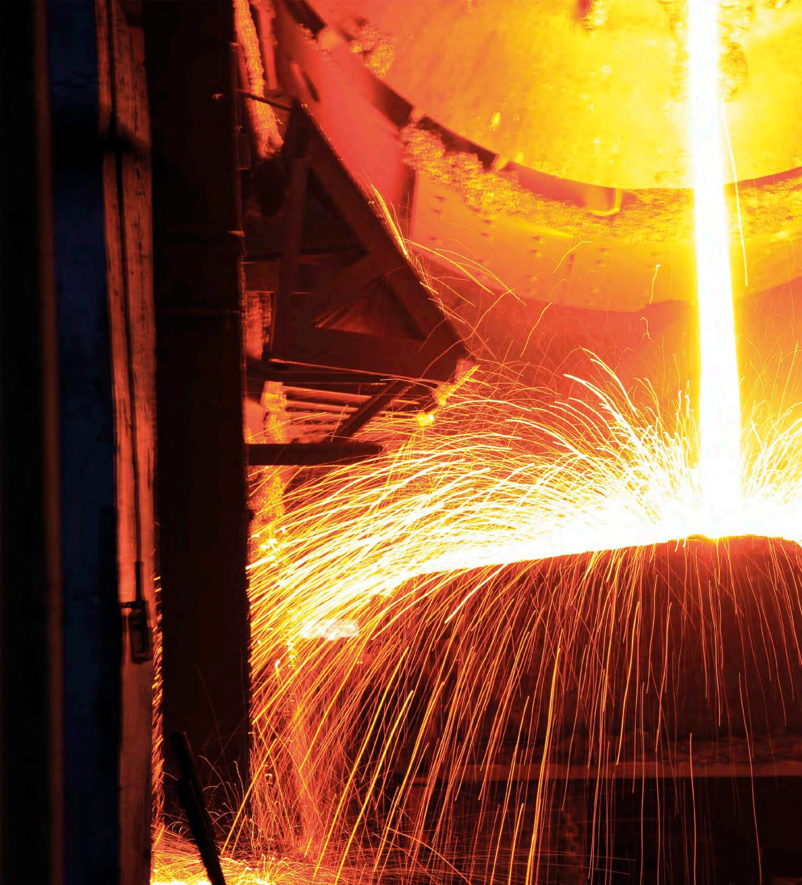
**STEELMAKING** A stream of red-hot, liquid metal pours from a furnace at a steelmaking workshop. This is the end of a long process in which iron ore is transformed into steel, a tough alloy that is strong enough to make girders for supporting skyscrapers and bridges. The steel may even be moulded into car bodies, woven into superstrong cables for elevators, or turned into powerful magnets that can levitate maglev trains.
