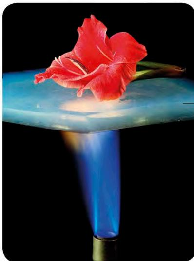
Silicate aerogel in an experiment
