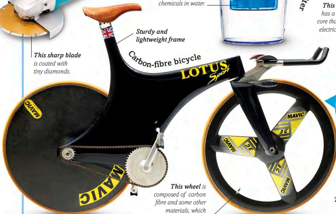
This **strong** but **light** frame is made by fusing together carbon fibres.
