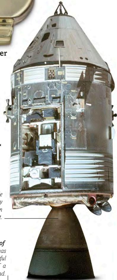
*This nozzle made of a niobium alloy kept its shape even when very hot.*
