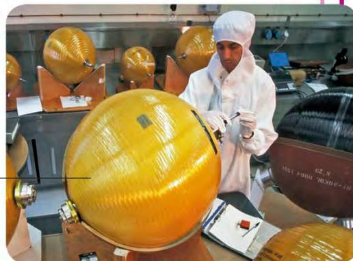
*Helium in this container will fill up a rocket's fuel tanks as they empty out during liftoff.*
