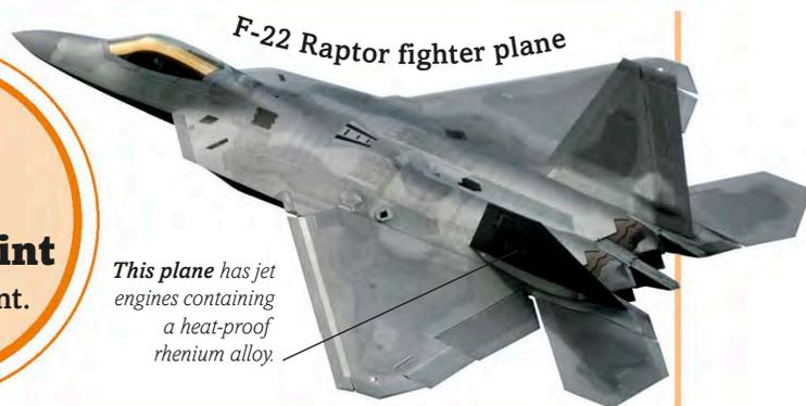
*This plane has jet engines containing a heat-proof rhenium alloy.*
