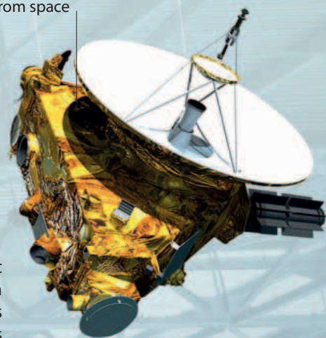
New Horizons instrument, called Ralph, provides heat maps and colour images from space
