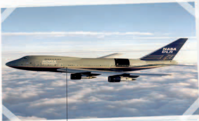
Aircraft houses a 2.5-m (8-ft) wide infrared telescope.
